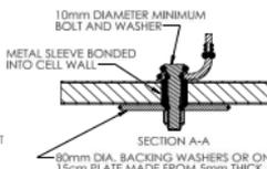
30mm DIA. BACKING WASHERS OR ONE 54mm x 15cm PLATE MADE FROM 5mm THICK ALUMINUM OR 4mm THICK STEEL (SEE WASHER OR PLATE SKETCHES)
