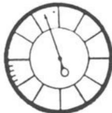
This clock is to be driven electrically or mechanically. It has only one hand moving continuously and indicating the seconds.
