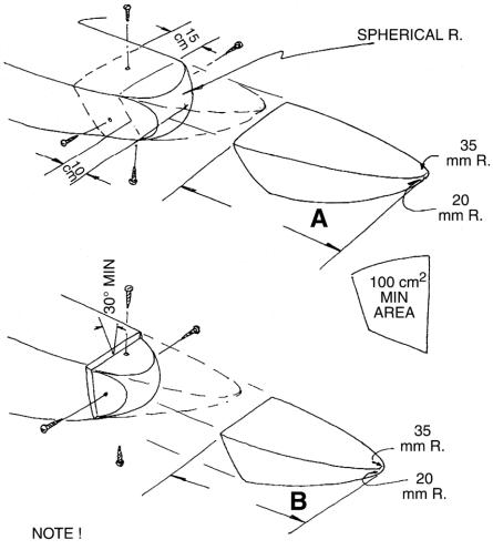
PICKLEFORK MUST DEFORM AT 100 kg MAXIMUM
