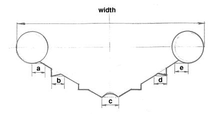
For PR 550, 700, 750, 850 : a+b+c+d+e < 10 % of the width For PR 1000, 1500, 2000, 3000 : b+c+d < 20 % of the width
