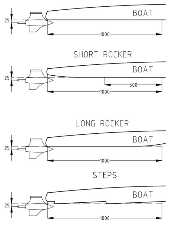
HYDROPLANE PROPELLER SHAFT HEIGHT MEASUREMENTS
