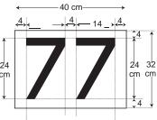
In case of a 3 digit numbers, the length of the surface must be modified consequently.
