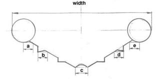
For PR 550, 700, 750, 850 : a+b+c+d+e < 10 % of the width For PR 1000, 1500, 2000, 3000 : b+c+d < 20 % of the width
