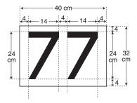
In case of a 3 digit numbers, the length of the surface must be modified consequently.
