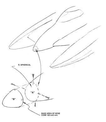
A. The front of cockpit must have the minimum radius as the front of the main body of the sponson, before the crushable picklefork.
