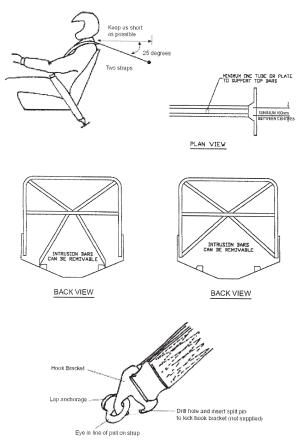
A split pin must lock the seat belt hook to the lap anchorage.
